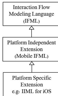
**Fig. 2.** Modeling languages stack: mobile IFML defined as a mobile extension of IFML shall be used to model the front-end of the app at the PIM level. The required PSM languages will be defined as extensions of the mobile IFML.
