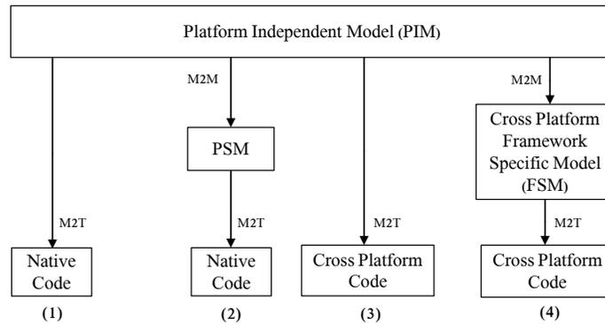
**Fig. 1.** MDD approaches for cross-platform mobile apps development: the requirements of the app are described in a PIM from which the app code is generated through the application of a set of model-to-model(M2M) and/or model-to-text (M2T) rules.
