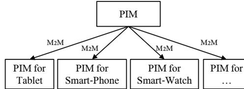
**Fig. 3.** Multi device development: The app requirements are described in a **general** PIM. Different model transformations are applied to that PIM to produce a new PIM that describes the shape of the app in each of the target device families. The M2M transformations can be conceptualized for instance through a set of ATL [11] rules
