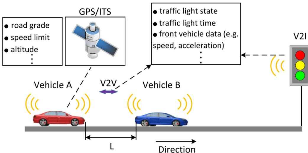
Figure 1: The scenario of two-vehicle energy management.
